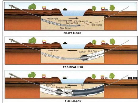
Figure 3. Figure 3. HDD operation (FHWA, 2013)
