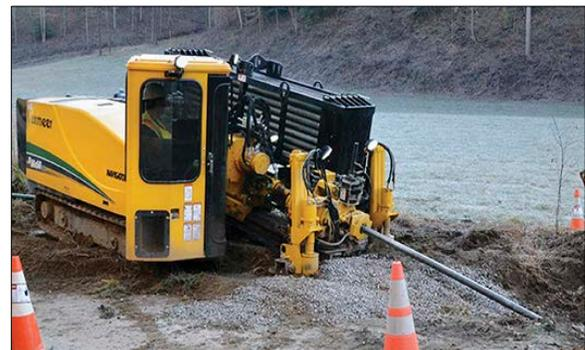
Figure 2. Figure 2. HDD rig during a pilot boring stage (Vermeer, 2015)
